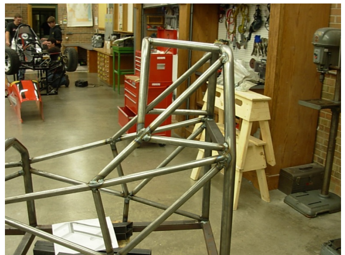
Halo bars installed on the frame
